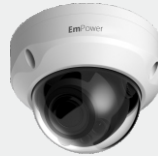
HC-2DM-MVF-PA Starlight, 120dB true WDR, 3DNR Max 30fps@1080P HD and SD output switchable 2.7-13.5mm motorized lens Max. IR length 30m, Smart IR IP67, IK10, AC24V/DC12V
