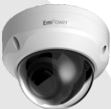
HC-4DM-VF-SA Max 30fps@4MP HD and SD output switchable 2.7-13.5mm vari-focal lens Max. IR length 30m, Smart IR IP67, IK10, DC12V
