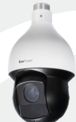
HC-2PT-5I2Z5A 1/2.8" 2Megapixel STARVIS™ CMOS Powerful 25x optical zoom Starlight technology 120dB true WDR, 3D DNR Max. 25/30fps@1080P, 25/30/50/60fps@720P IR distance up to 150m; IP66
