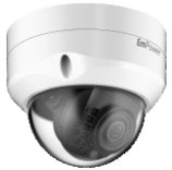
HC-2DM-F36-SA Max 30fps@1080P HD and SD output switchable 3.6mm fixed lens Max. IR length 30m, Smart IR IP67, IK10, DC12V
