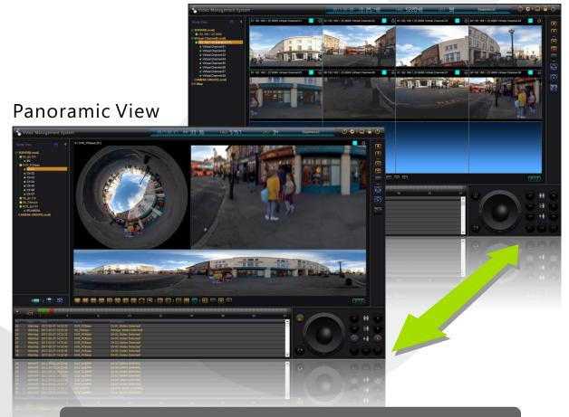
Fisheye cameras are now a standard video device. With our universal **360° Panorama** the **Unisight Client** module can dewarp any fisheye camera, regardless of manufacturer, when mounted on the wall or ceiling and even on the roof/ground for aerial surveillance.
